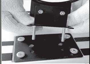
1) Insert the screws Part I into holes of Breakaway Rim Part B.
