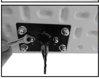
3) Using wrench to tighten the nuts on back of board.(Wrench not provided)
